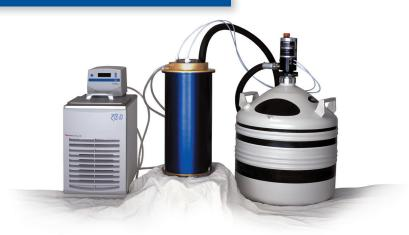
Calibration standards based on the primary physic constants of thermal noise and blackbody radiation. This provides the ultimate accuracy when measuring extremely low noise figures (noise temperatures). Simple, and versatile to use, the NBS-Series is an ideal solution for noise source calibrations, radiometer test references and low noise amplifier tests.
