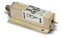
Excellent choice for applications requiring high ENR and immunity to large incident RF power found in radiometer and radar systems. The calibration accuracy and flatness of the NC3400 Series noise sources are enhanced by their low VSWR. The built-in isolator provides almost constant output impedance as the noise source bias is switched on and off. The isolator also protects the noise diode from incident RF power (consult the factory for high power units).
