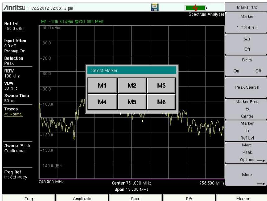
**Figure 2-12.** Select Active Marker with the Touch Screen
