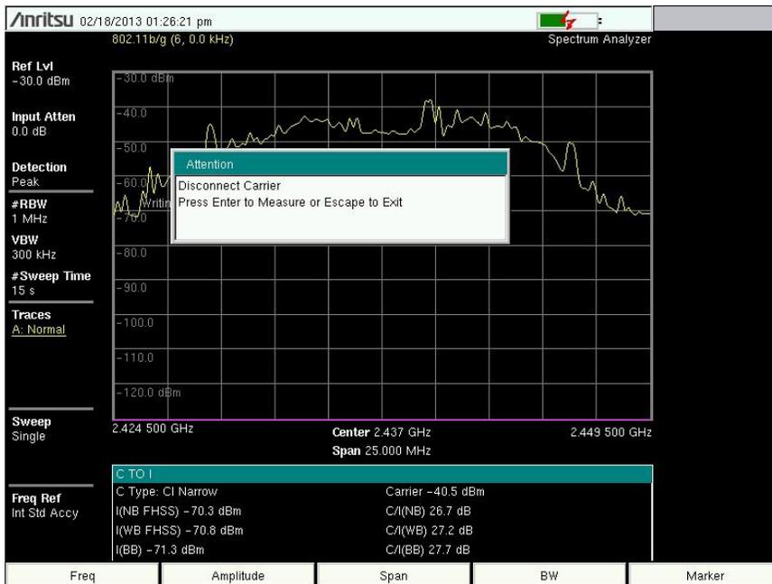
Figure 2-15. C/I Measurement, Carrier Measured
