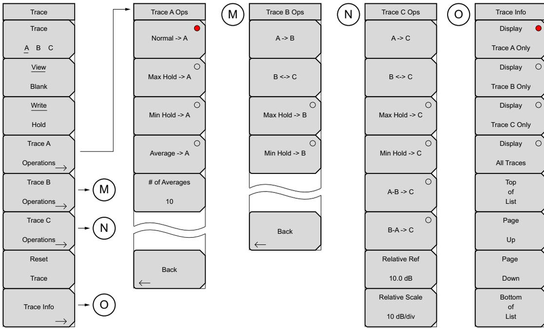
Figure 2-33. Trace Submenu Keys
