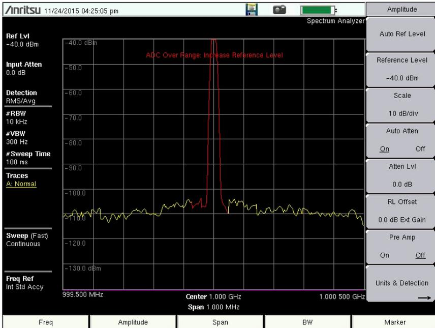
Figure 2-6. ADC Over Range - On Screen
