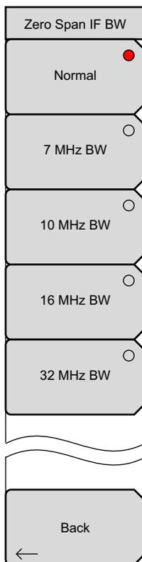
**Figure 2-2.** Zero Span IF Bandwidth Selection Menu
