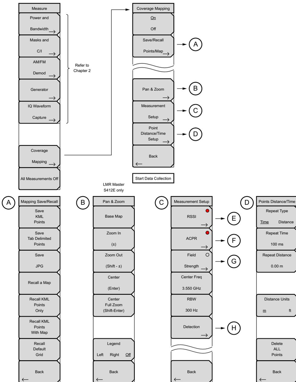
Figure 6-7. Coverage Mapping Menu Keys
