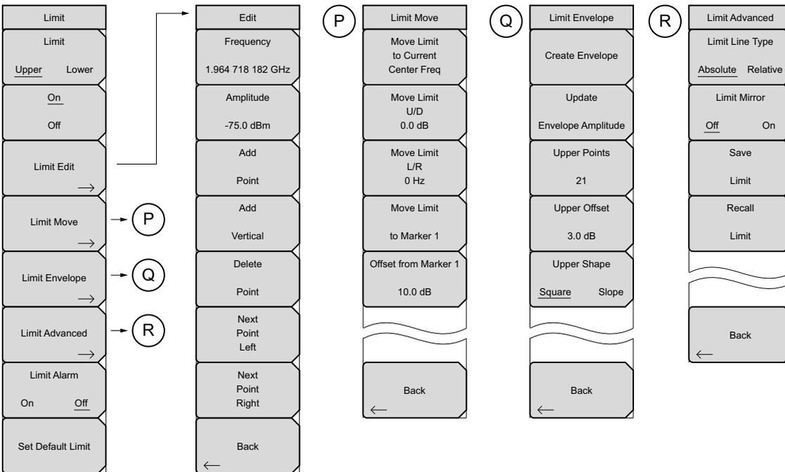
Figure 2-34. Limit Submenu Keys
