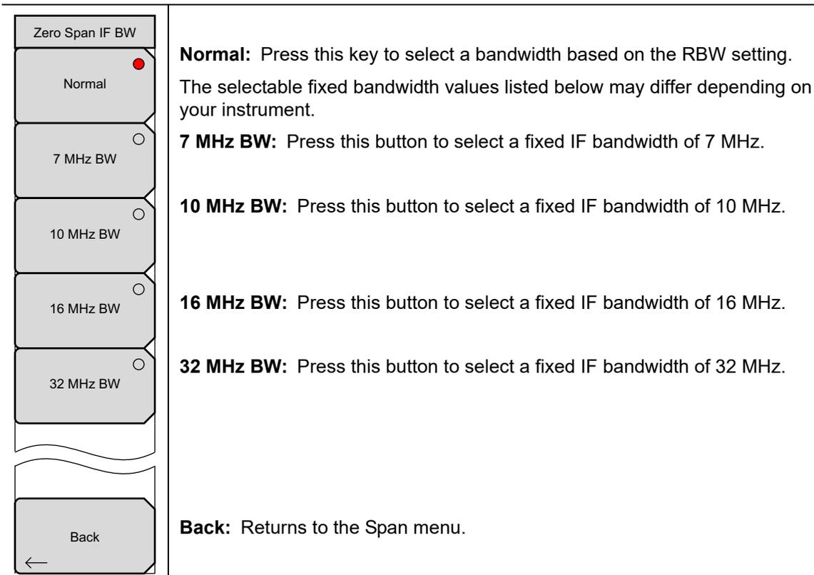
**Figure 2-44.** Zero Span IF BW Menu
