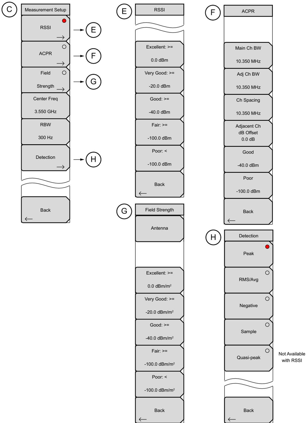
Figure 6-8. Coverage Mapping Menu Keys (Part 2)
