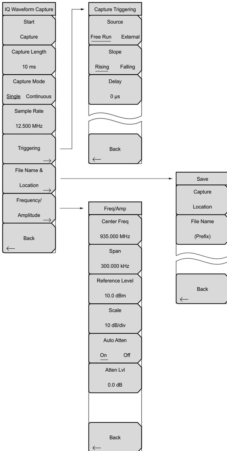
Figure 3-18. IQ Waveform Capture Submenu Keys (Option 24)
