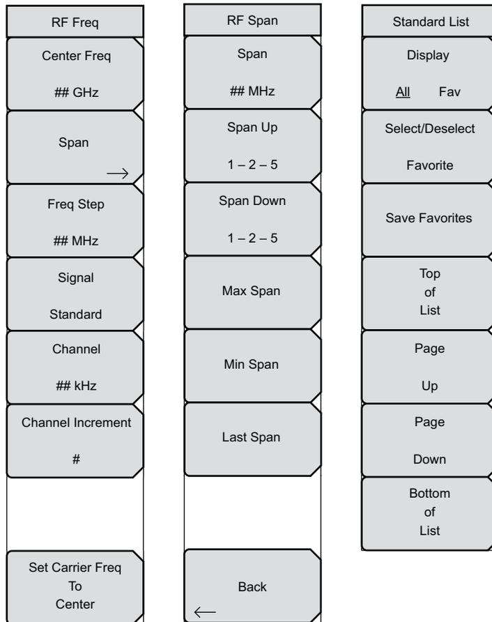
**Figure 7-6.** Frequency Menu with AM/FM/PM Analyzer (Option 509)
