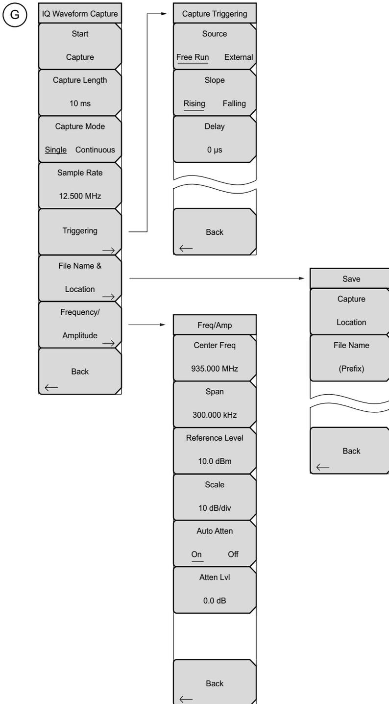
Figure 2-31. IQ Waveform Capture Submenu Keys (Option 24)
