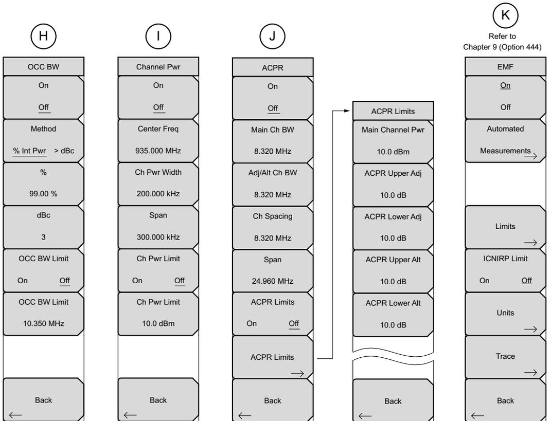
Figure 2-28. Measure Submenu Keys — Power and Bandwidth
