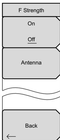
This measurement allows the use of an antenna with known gain characteristics and measures the field strength over the frequency range of the antenna in units of dBm/m<sup>2</sup>, dBV/m, dBmV/m, dBμV/m, Volt/m, Watt/m<sup>2</sup>, dBW/m<sup>2</sup>, A/m, dBA/m, or Watt/cm<sup>2</sup>.
