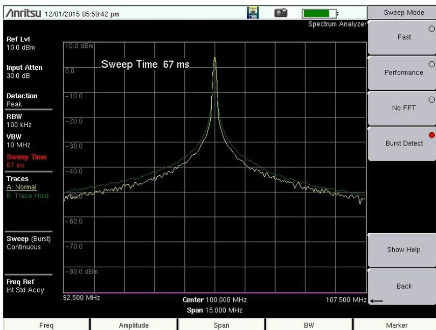
Figure 2-1. Example of Burst Detect Sweep Mode
