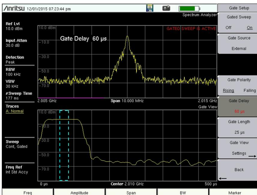
**Figure 2-3.** Gated Sweep Example - External Gate Source
