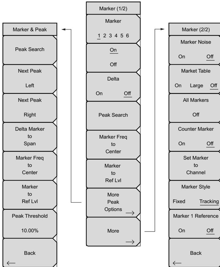
Figure 2-26. Marker Submenu Keys
