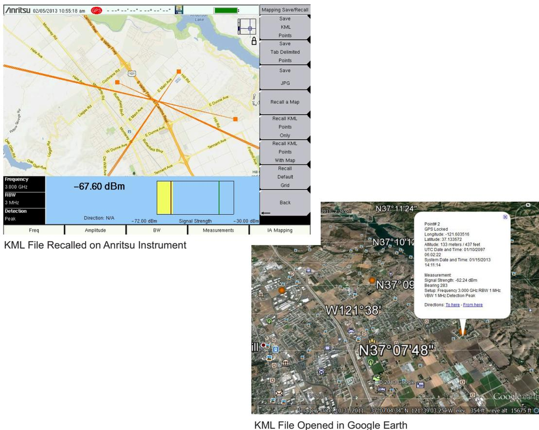
Figure 3-12. KML File on the PC and the Anritsu Instrument
