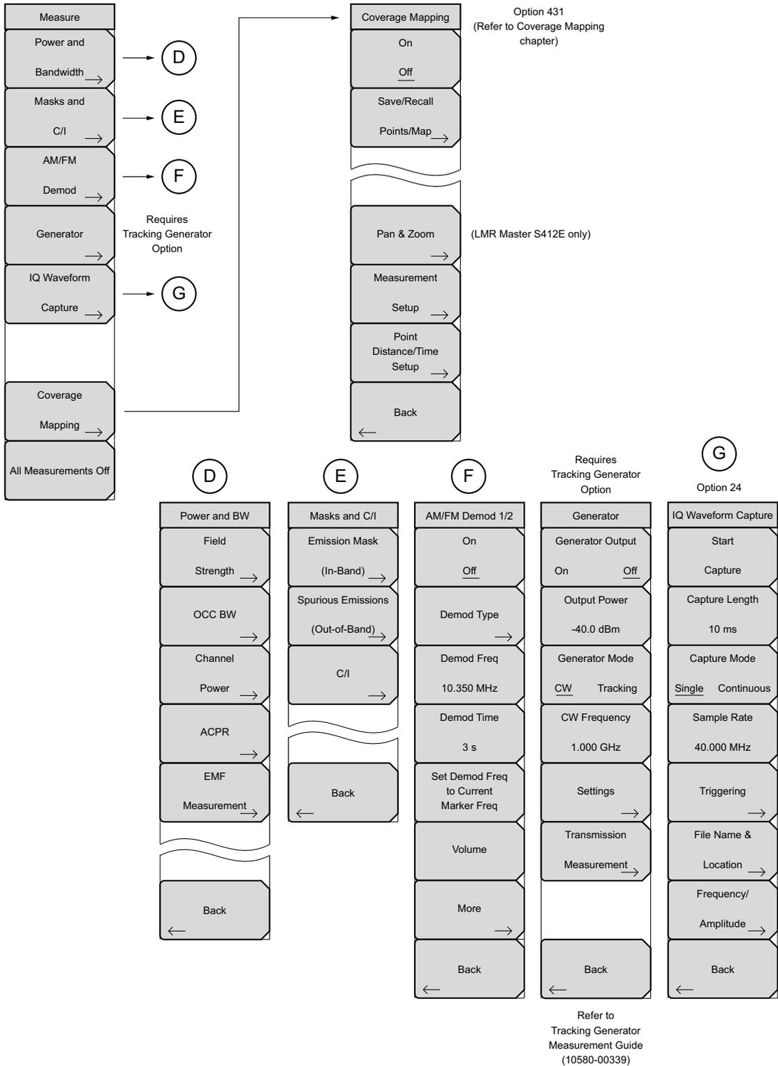
Figure 2-27. Measure Submenu Keys — Measure
