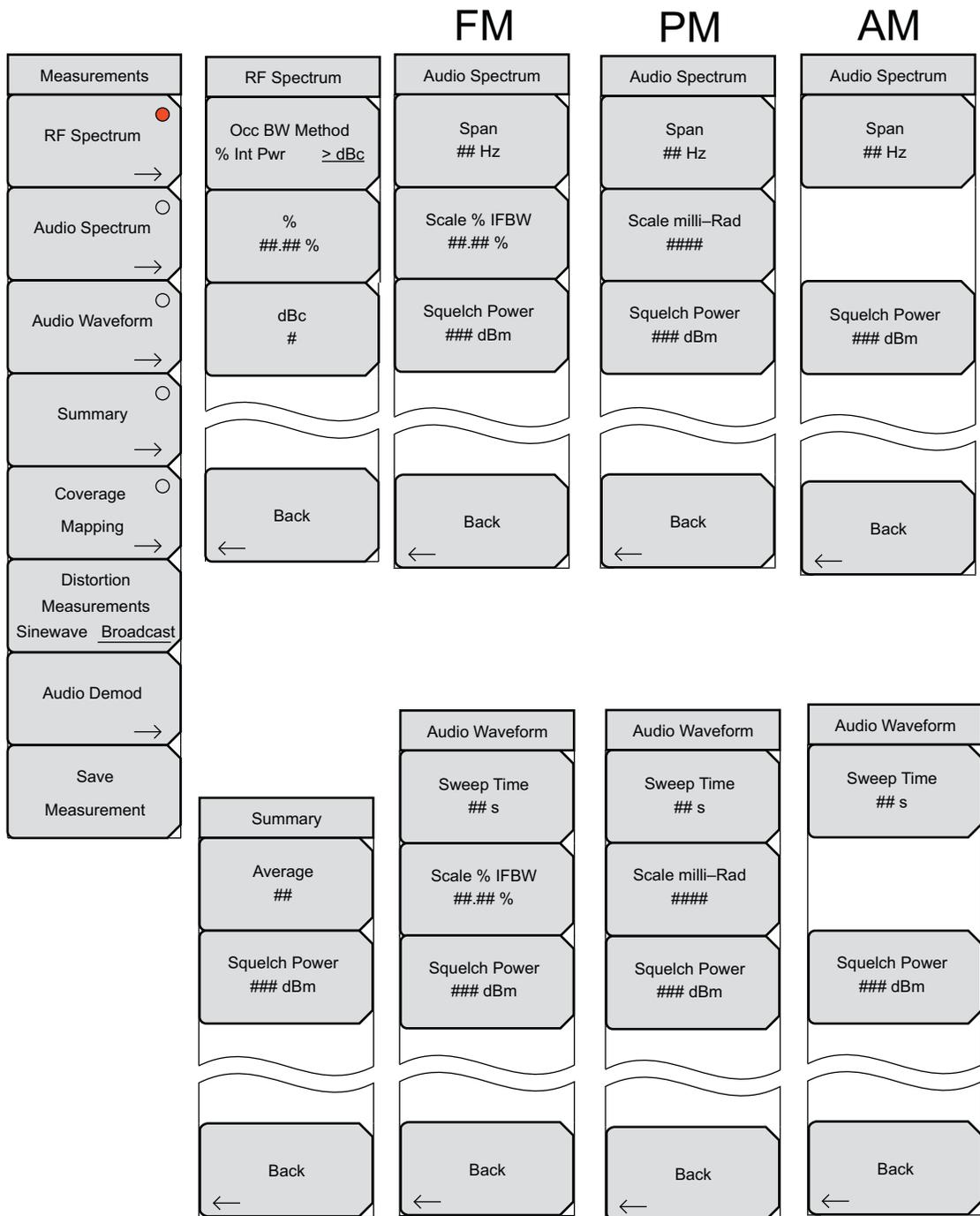
Figure 7-7. Measurements Menus with AM/FM/PM Analyzer (Option 509)
