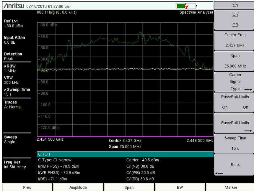
Figure 2-16. C/I Measurement, Results
