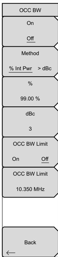
**On/Off:** This submenu key turns the Occupied Bandwidth On or Off.
