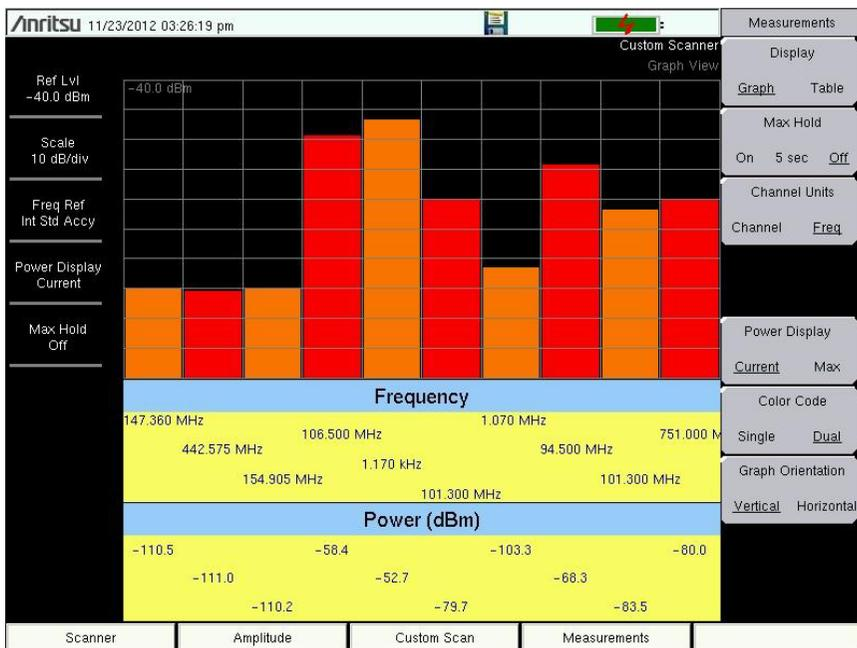
Figure 4-9. Channel Scanner Graph Display with Vertical Orientation
