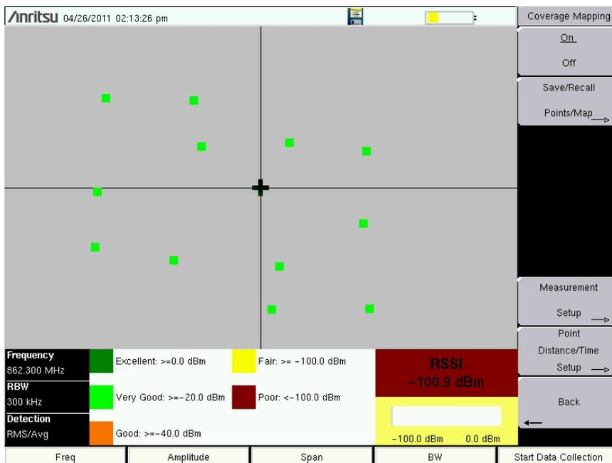
Figure 6-3. Coverage Mapping with the Default Grid.
