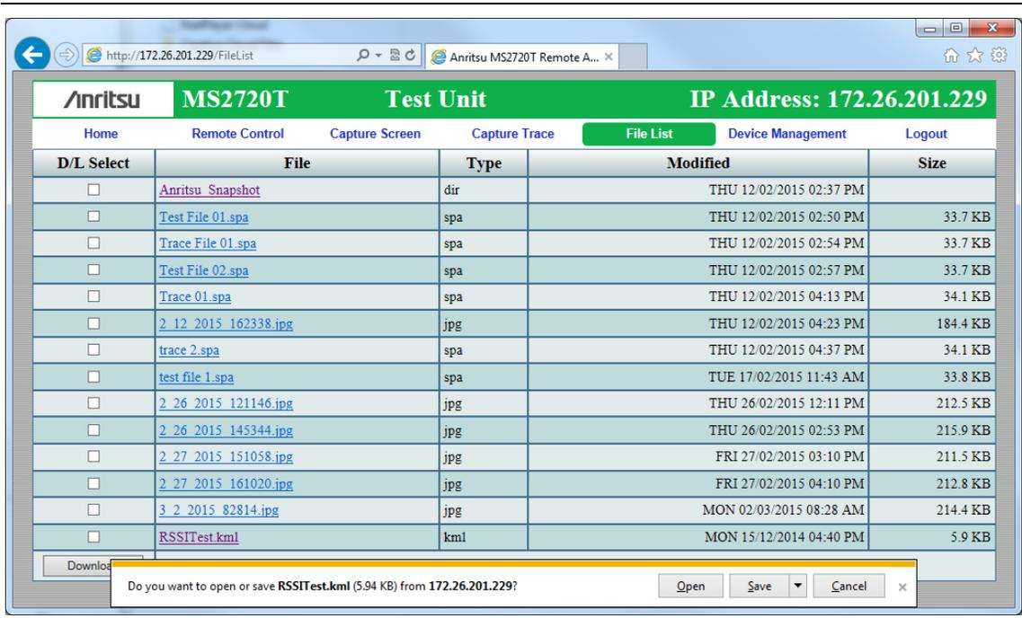
Figure 6-4. Web Remote Control Window - File List Tab
