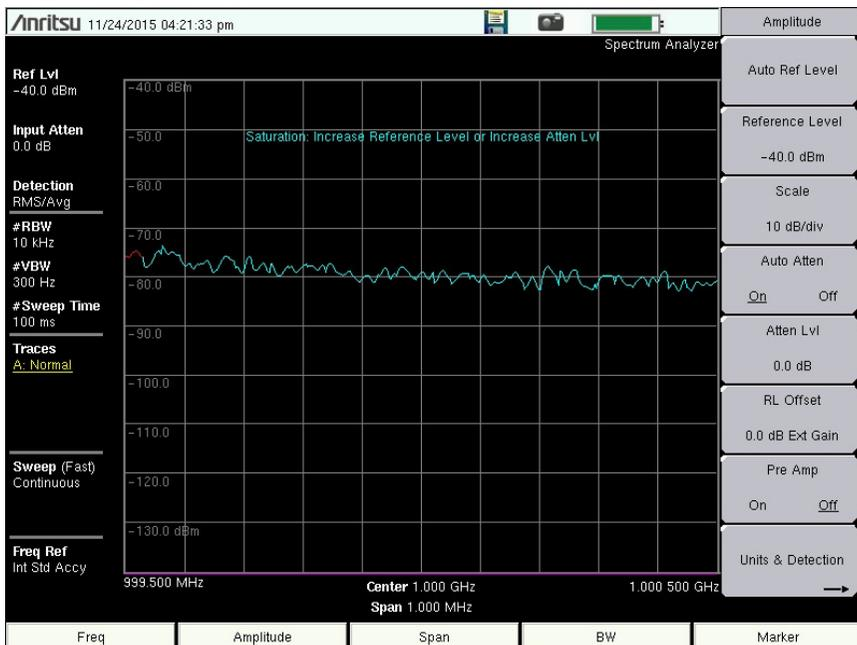
Figure 2-5. Saturation - Off Screen
