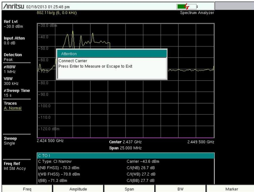
Figure 2-14. C/I Measurement, Ready to Measure the Carrier
