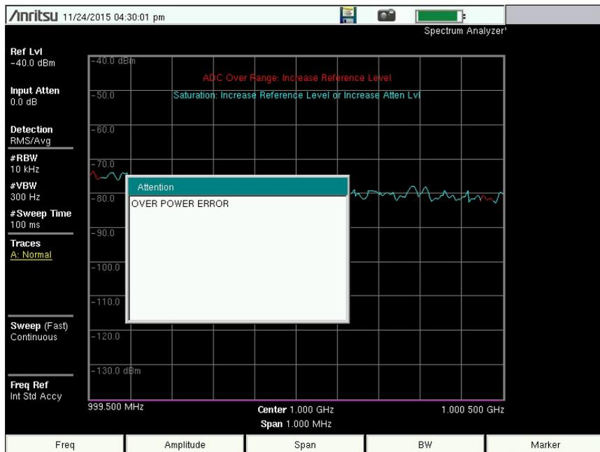
Figure 2-8. Over Power Error (MT8220T and MS2720T-0709 only)
