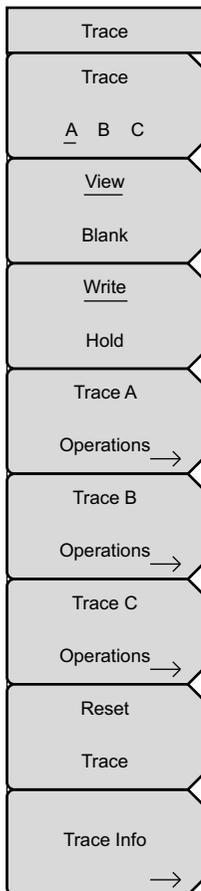
**Trace A, B, C:** Sets trace A, B, or C as the active trace. Repeatedly pressing this key toggles through trace A, B, and C. The active trace is underlined.
