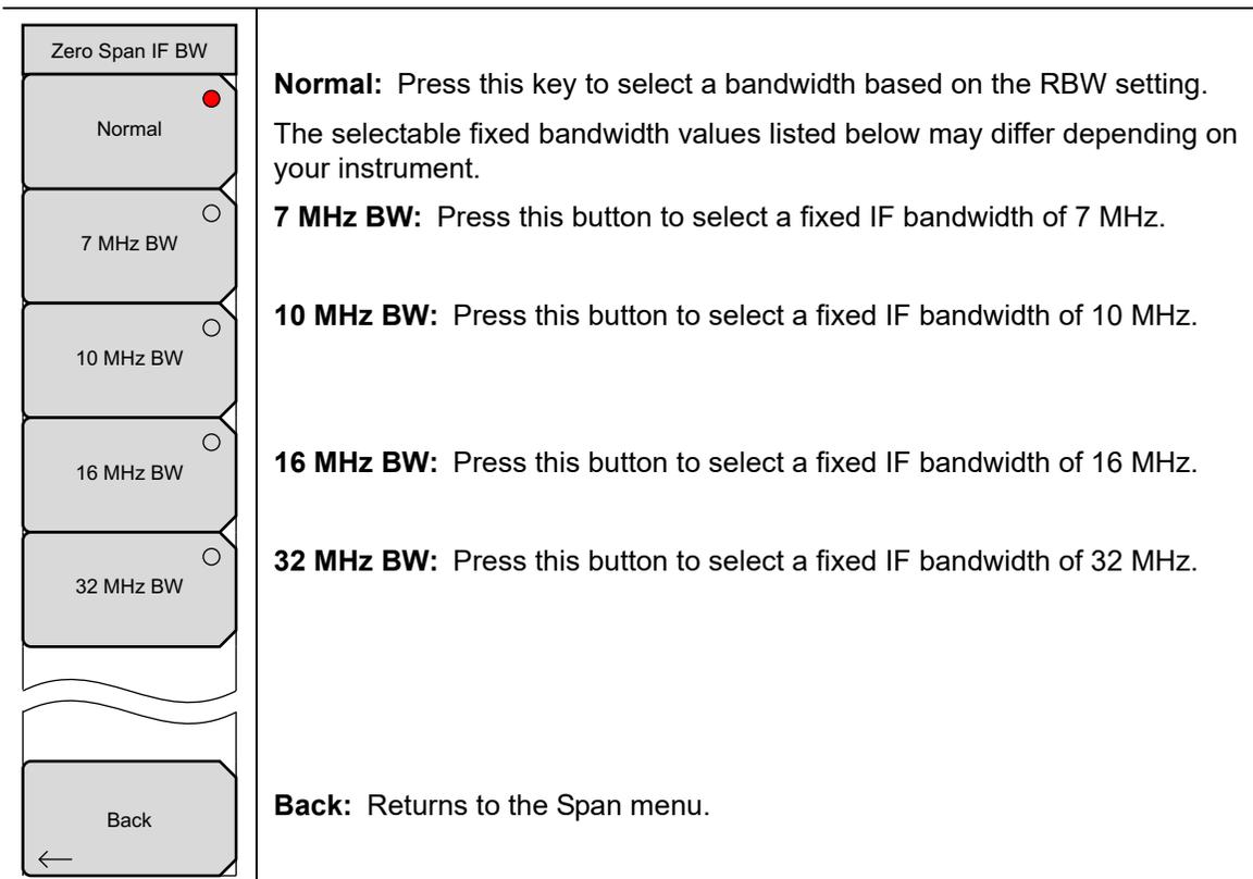
**Figure 3-30.** Zero Span IF BW Menu
