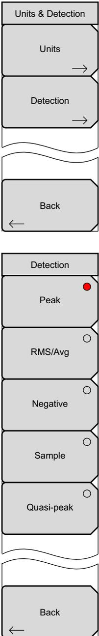
**Units:** Press this submenu key to select the amplitude unit: dBm, dBV, dBmV, dBμV, Volt, Watt, dBW, Amp, or dBA. When measuring Field Strength, values may be displayed in dBm/m<sup>2</sup>, dBV/m, dBmV/m, dBμV/m, Volt/m, Watt/m<sup>2</sup>, dBW/m<sup>2</sup>, A/m, dBA/m, or Watt/cm<sup>2</sup>. See [Figure 3-14 on page 3-22](#). Press Back to return to the Amplitude menu.
