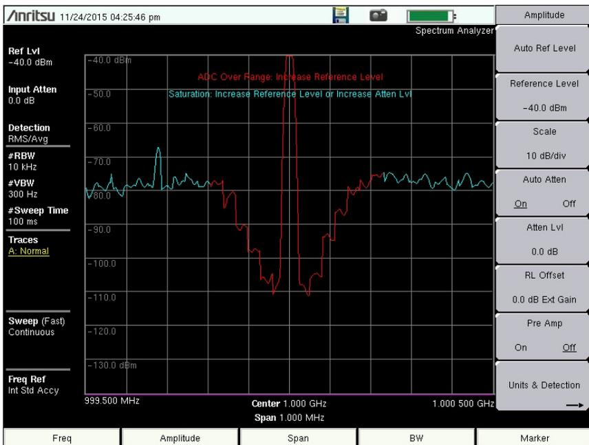
Figure 2-7. Saturation and ADC Overload
