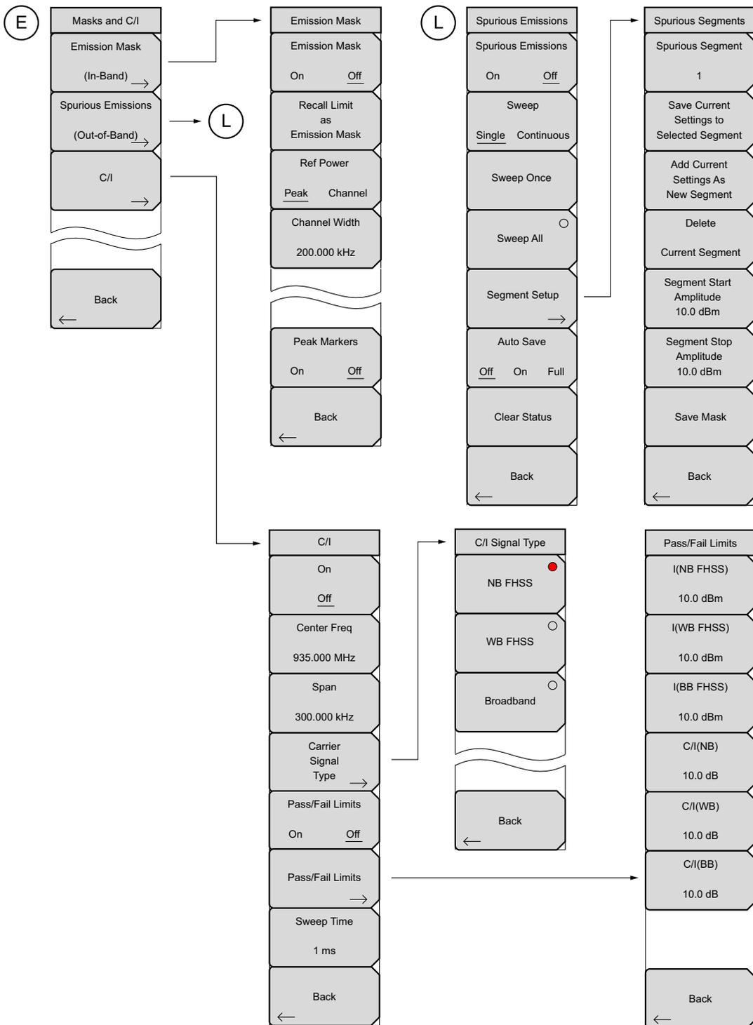
Figure 2-29. Measure Submenu Keys — Masks and C/I
