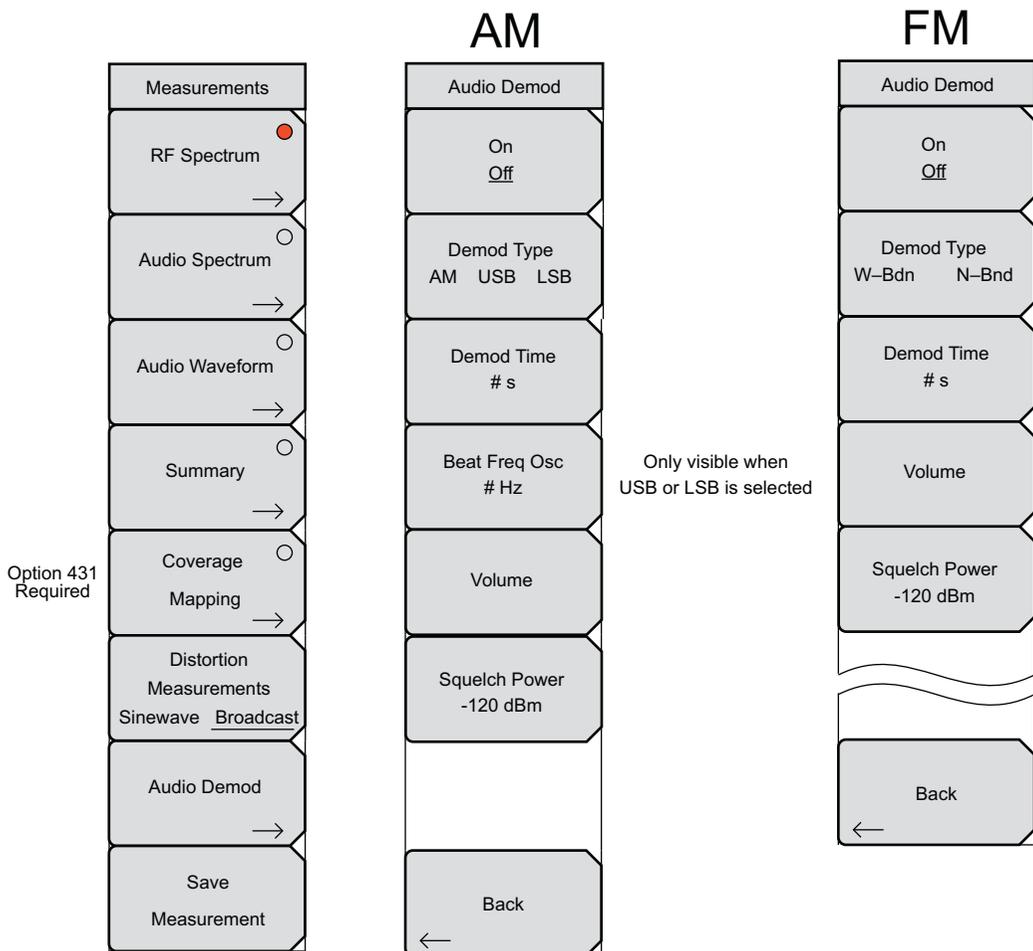
Figure 7-8. Audio Demod Menus with AM/FM/PM Analyzer (Option 509)
