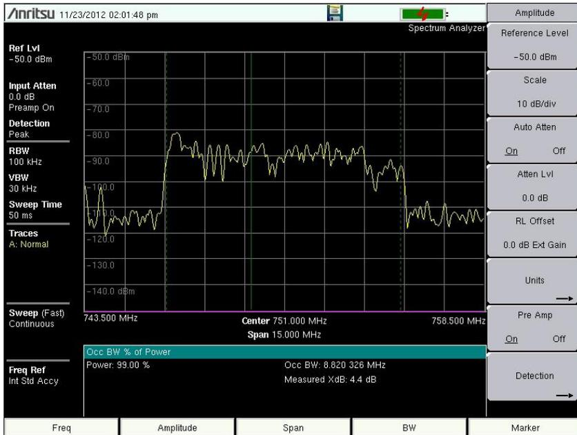
Figure 2-11. Occupied Bandwidth Results Using the % of Power Method
