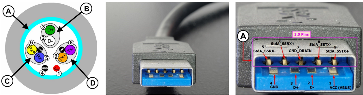
Figure 12-81: USB 3.1 cable cross-section and Standard-A plug - backward compatible with USB 2.0
