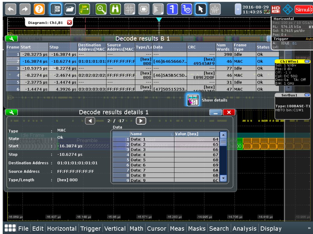
Figure 12-45: 100BASE-T1 decode results table and details
