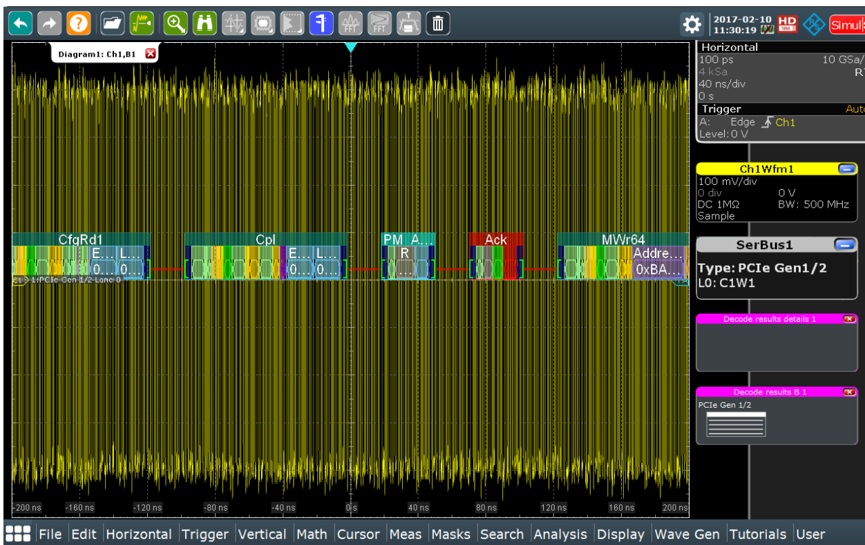
Figure 12-93: PCIeGen 1/2 protocol: decoded and binary signal
