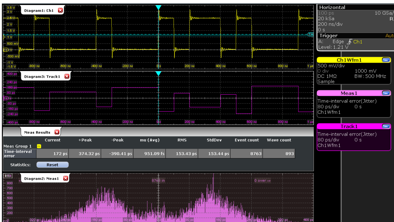
Figure 16-1: TIE measurement with CDR trigger, 10 Mbps, with track and histogram
