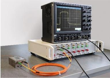
Montena MOL2000T optical link is designed for the transmission of analogue electric signals (CW and pulses) from 80 Hz to 3.5 GHz over long distance in harsh electromagnetic environment.
