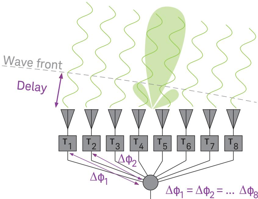
Lock up to 16 PSG vector signal generators to achieve phase coherency with special Option HCC
