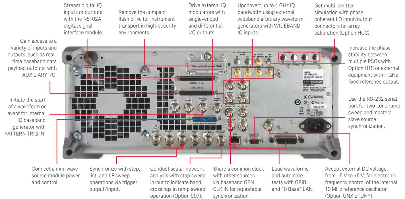
Note: Available connectors vary depending on the PSG model and option structure configuration
