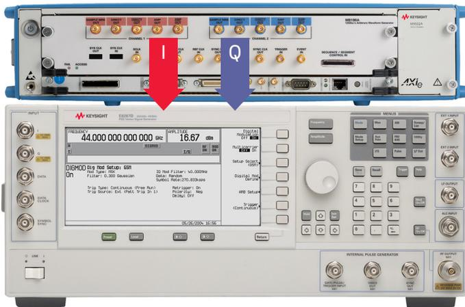
Simulate simultaneous multiple emitters with up to 4 GHz modulation bandwidth using E8267D, M8190A AWG, and external IQ inputs Option 016
