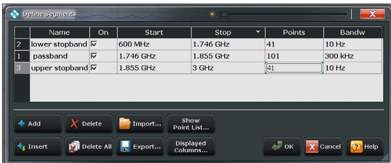
Filter measurement using segmented sweep.
