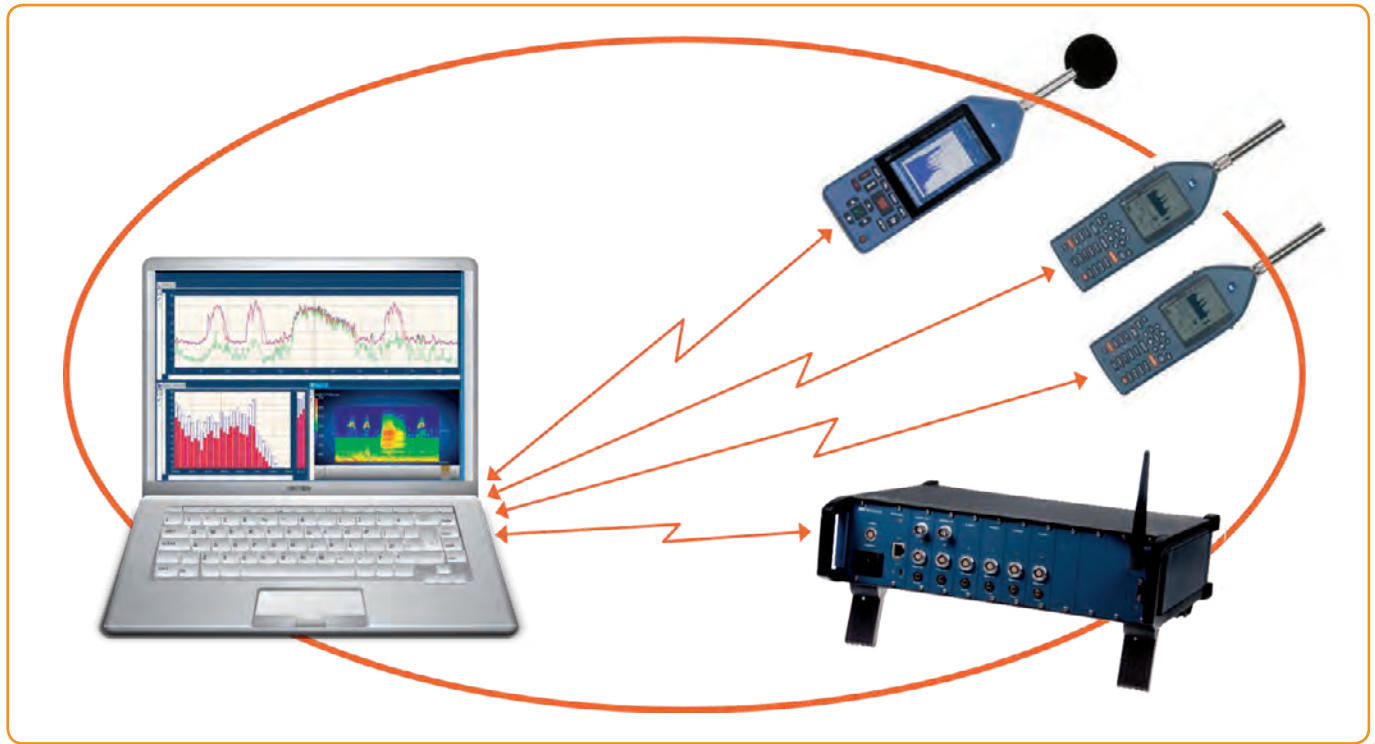
Nor850 is a distributed multi-channel measurement system
