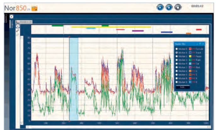
Measurement markers along the upper time-axis
