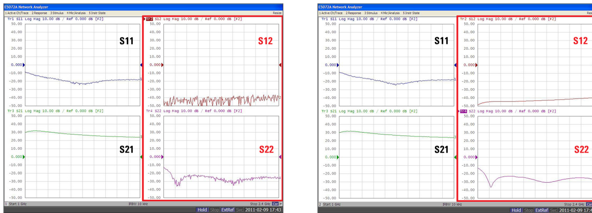
Coupled power (Port 1 = Port 2 = -40 dBm)
