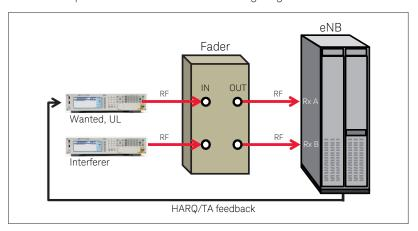
In Signal Studio, real-time mode is used to define the parameters of nonrepeating signals needed for receiver testing. Its graphical interface provides a direct instrument connection for parameter transfer and closed-loop or interactive control during signal generation. Real-time capabilities are currently available in versions of Signal Studio that address the following standards:
