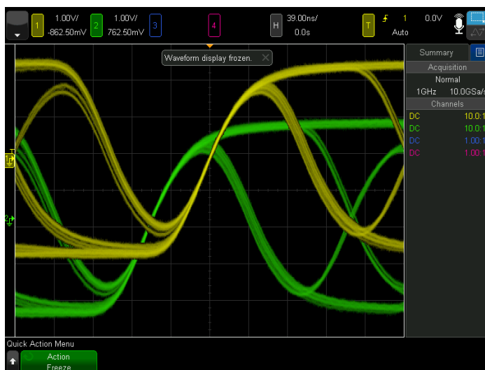
Figure 54. Quick Freeze Display preserves the persistence.
