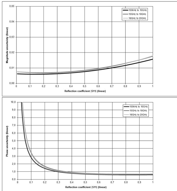
Typical accuracy of reflection magnitude and reflection phase measurements for the R&S®ZNBT20 in the frequency range from 100 kHz to 20 GHz, calibrated with a ZV-Z235 calibration kit that has been characterized with a DAkkS-accredited calibration. Analysis conditions:  $S_{12} = S_{21} = 0$ , cal. power -10 dBm, meas. power -10 dBm.
