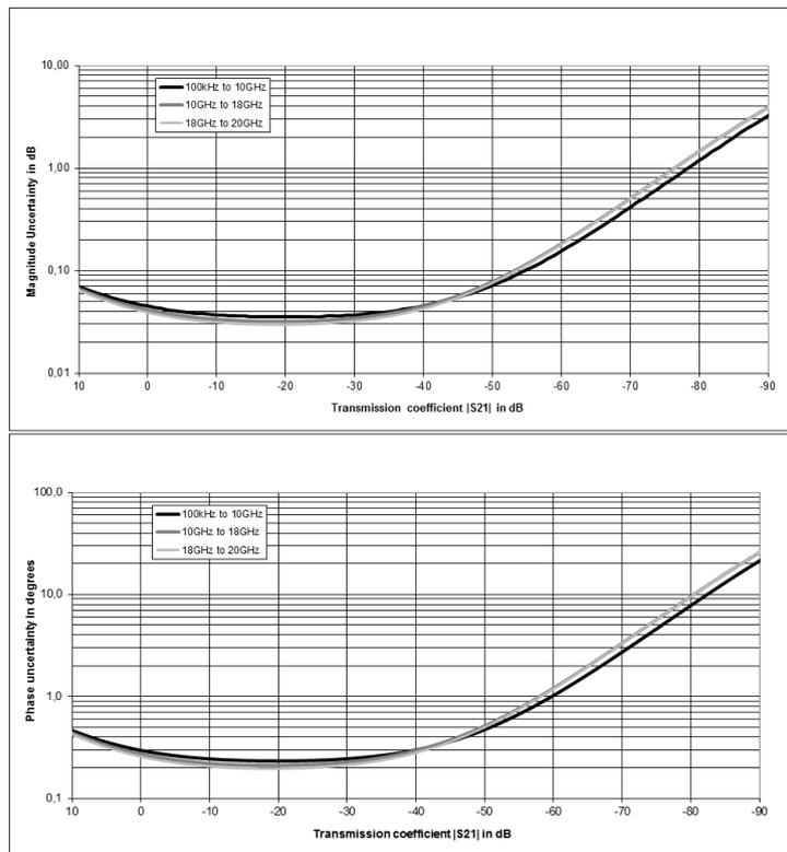
Typical accuracy of transmission magnitude and transmission phase measurements for the R&S®ZNB20 in the frequency range from 100 kHz to 20 GHz. Analysis conditions:  $S_{11} = S_{22} = 0$ , cal. power -10 dBm, meas. power -10 dBm.
