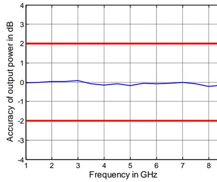
Output power accuracy in dB versus frequency for the R&S<sup>®</sup>ZNBT8.
