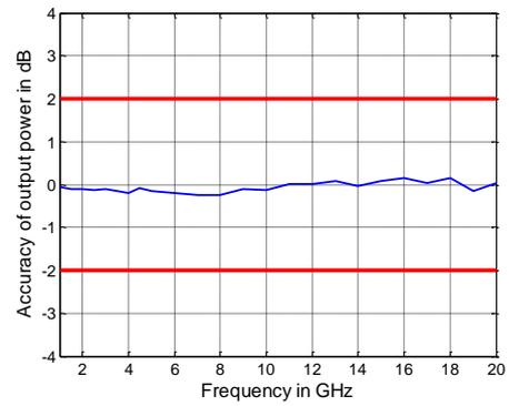
Output power accuracy in dB versus frequency for the R&S<sup>®</sup>ZNBT20.
