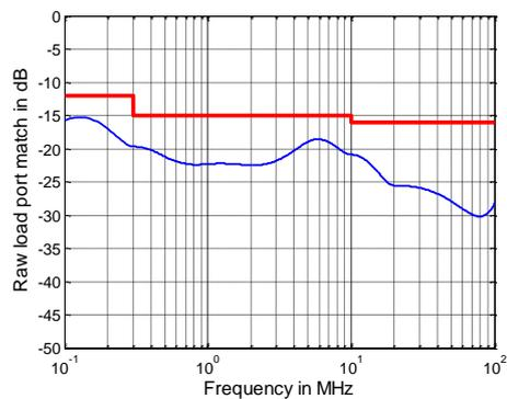
Raw load port match versus frequency for the R&S®ZNBТ20.
