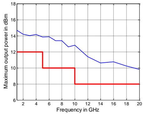
Maximum output power in dBm versus frequency for the R&S<sup>®</sup>ZNBT20.
