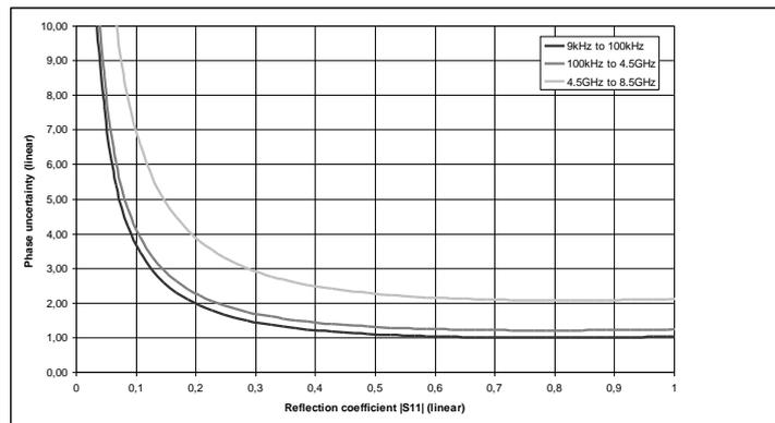
Typical accuracy of reflection magnitude and reflection phase measurements for the R&S®ZNB T8 in the frequency range from 9 kHz to 8.5 GHz. Analysis conditions:  $S_{12} = S_{21} = 0$ , cal. power -10 dBm, meas. power -10 dBm.
