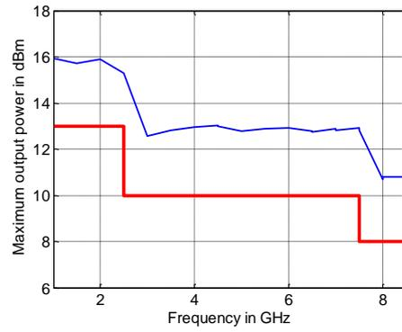
Maximum output power in dBm versus frequency for the R&S<sup>®</sup>ZNBT8.
