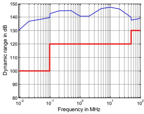
Dynamic range in dB versus frequency for the R&S<sup>®</sup>ZNBT8.
