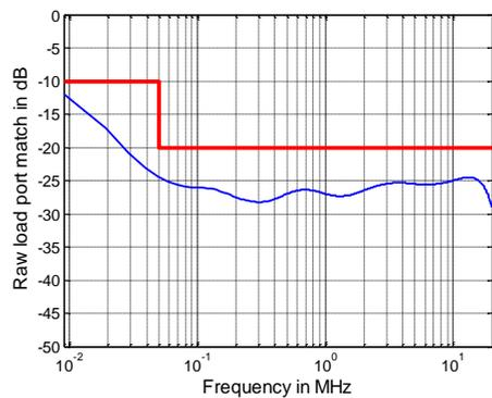
Raw load port match versus frequency for the R&S®ZNBТ8.
