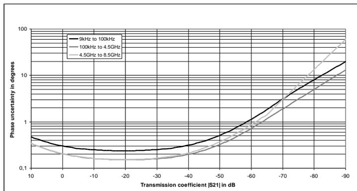
Typical accuracy of transmission magnitude and transmission phase measurements for the R&S®ZNB T8 in the frequency range from 9 kHz to 8.5 GHz.
