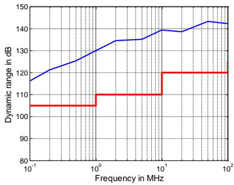
Dynamic range in dB versus frequency for the R&S<sup>®</sup>ZNBT20.
