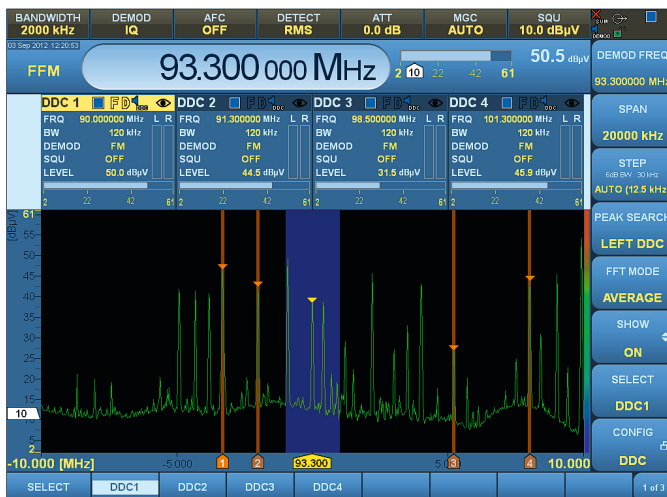
4+1 demodulation channels with different parameters within the realtime bandwidth.
