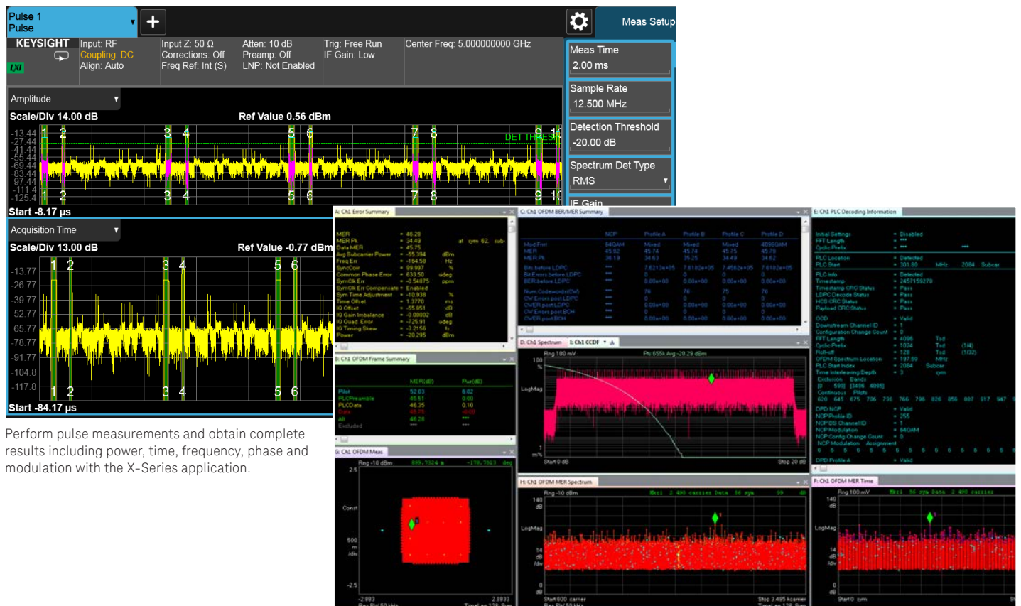
Use 89600 VSA software to gain deeper insights of DOCSIS 3.1 downstream signals through MER/BER summaries, PLC decoding information, and peak MER traces on the constellation, subcarrier and symbol domains.
