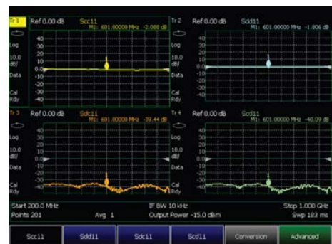
Characterized common and differential mode reflections with mixed-mode S-parameter measurements
