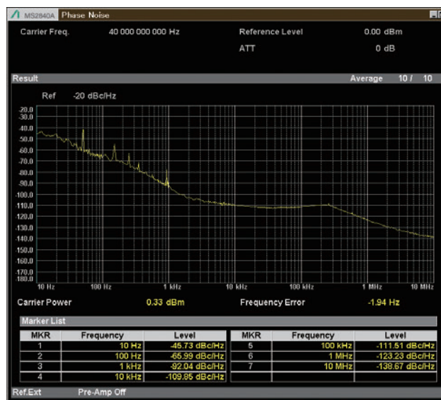
Phase Noise Measurement 40 GHz Measurement Frequency, Preamp Off
