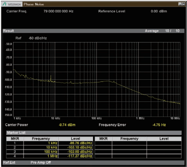
Phase Noise Measurement 79 GHz Measurement Frequency (Using High-Performance Waveguide Mixer MA2808A)
