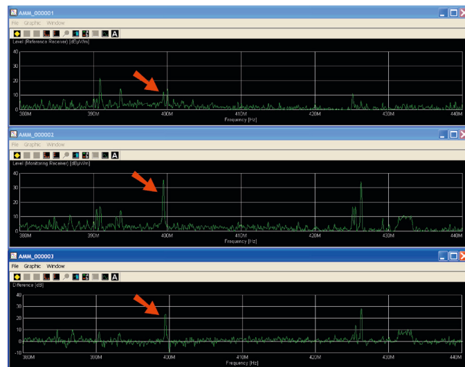
Display of differences in signal levels using the differential spectrum.
