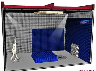
The Hermes 3 is designed to perform full-compliance emission and immunity tests at 3m distance on commercial equipment. The design of the structure is optimised for maximum performances, in minimum space. The shielding and its pyramidal absorbers are manufactured by SIEPEL.
