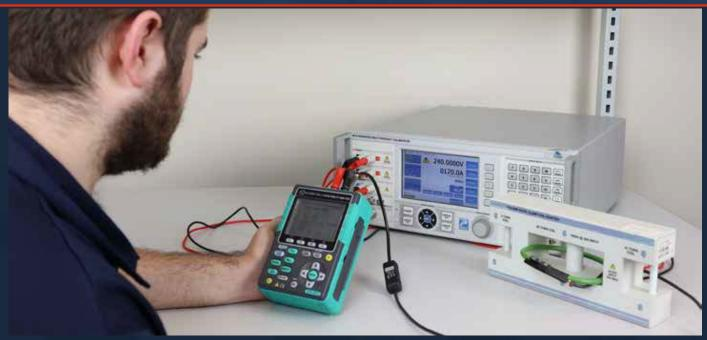
Included in -SYS units as standard, the PWRSINE option for the 4000 Series enables calibration of power meters, offering DC power output and AC power with variable phase between Voltage and Current outputs. Dynamic phase control enables calibration of both capacitive and inductive loads without additional error.
