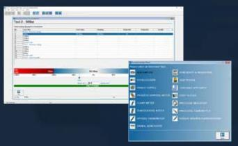
ProCal simplifies the task of calibration by providing a graphical interface with clear indication of test status using a 'Traffic light' system, where Green indicates pass, Red indicates a fail and orange indicates a probable fail or probable pass condition.
