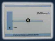
Using a high intensity LED light source, optical tachometers can be calibrated quickly and easily. Simply enter the RPM value using the calibrator keypad or use with ProCal software for automated calibration. With a range of 60 - 60,000 RPM the EA003 can be used to calibrate a wide range of optical tachometers.
