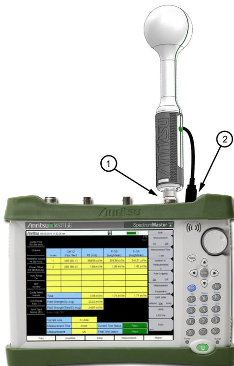
**Figure 3-1.** Connecting the Anritsu Isotropic Antenna
