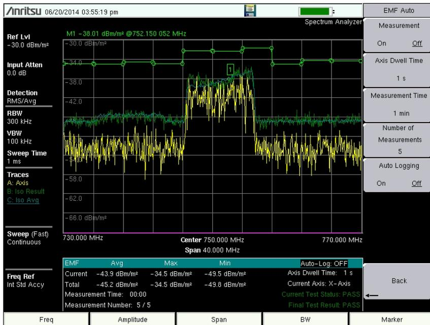
Figure 2-6. EMF Test Pass/Fail Status
