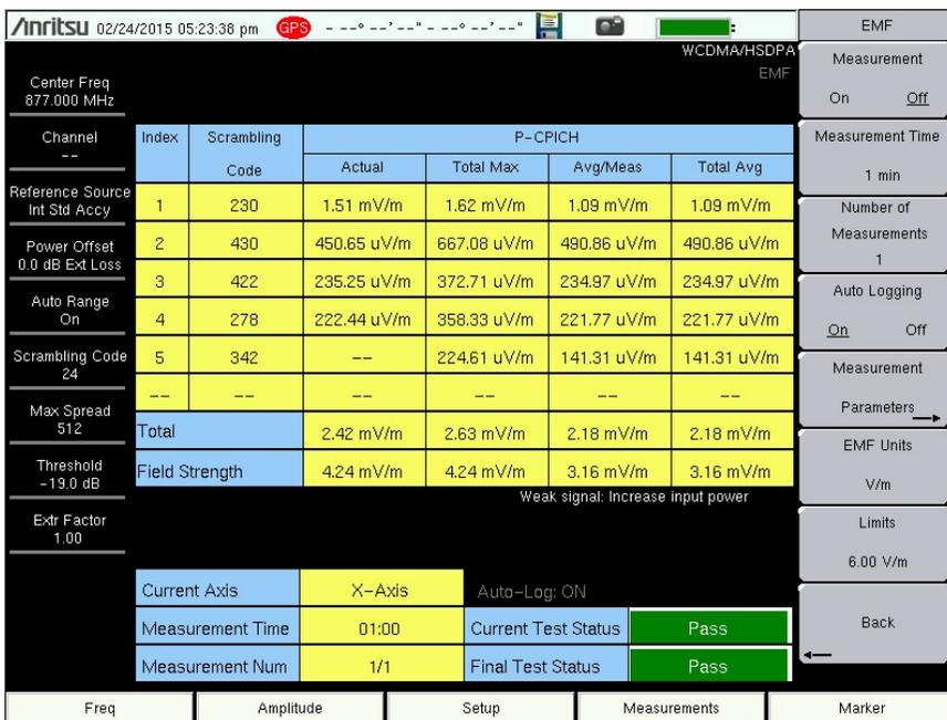
**Figure 4-6.** W-CDMA EMF Measurement Results
