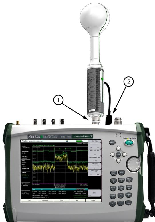
**Figure 2-1.** Connecting the Anritsu Isotropic Antenna
