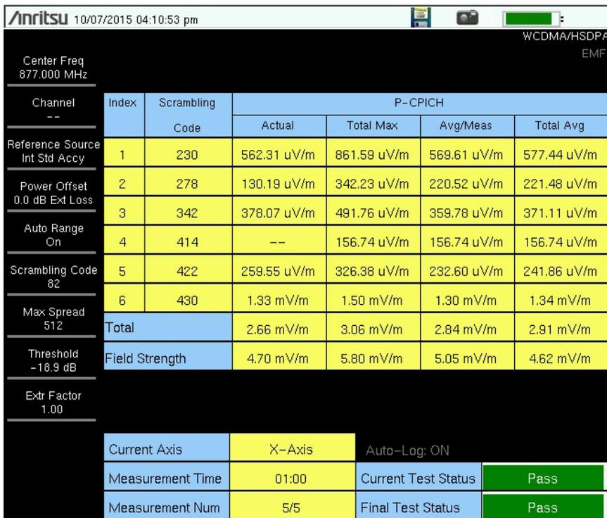
Figure 4-7. W-CDMA EMF Measurement Display
