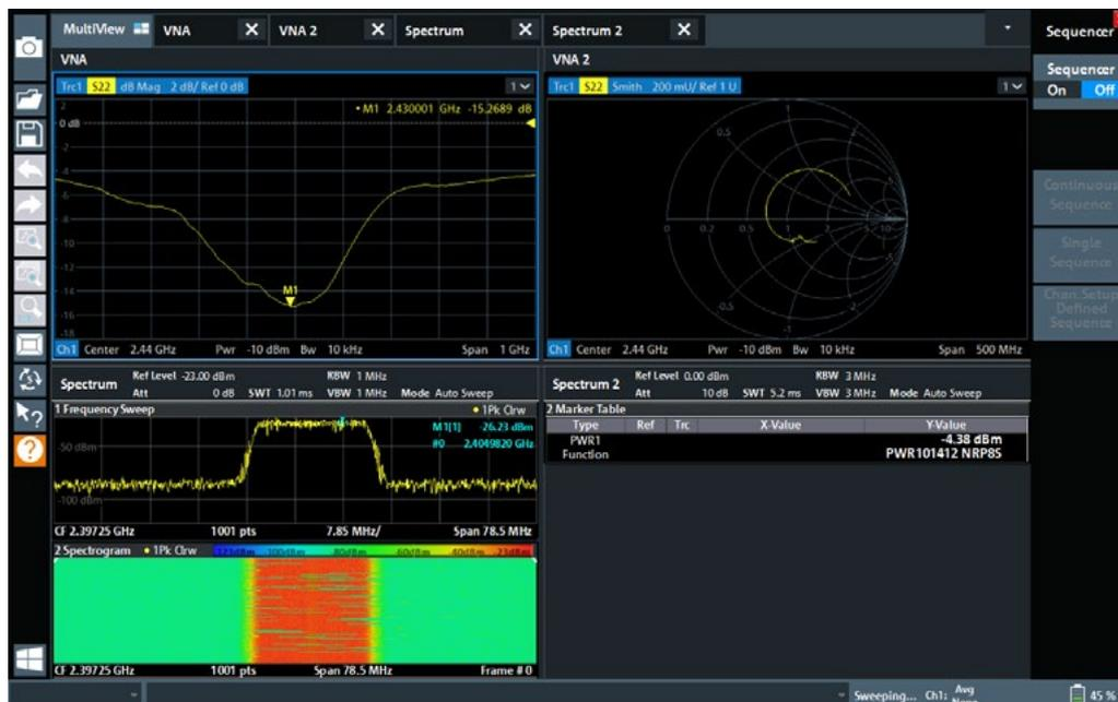
In MultiView all tabs can be seen at the same time. In this case one can see a VNA mode measurement in parallel to a SA mode measurement.
