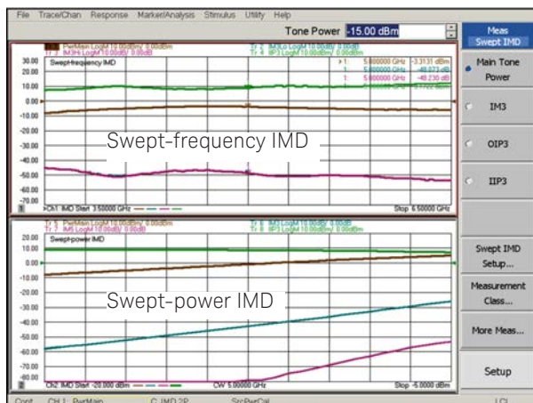
IMD application measures third order IMD and IP3 at 201 frequency (or power) points in a matter of seconds, compared to several minutes using signal generators and a spectrum analyzer.
