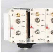
The compact optical receiver for multilink application is a plugin module. To be inserted in the MOL-MF-10 chassis.
