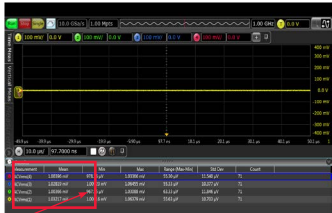
Figure 6. See how much noise your scope has. Disconnect inputs from the scope and measure noise (Volts RMS) at each vertical setting. In this example, each channel shows equal noise of just 1 mVrms.
