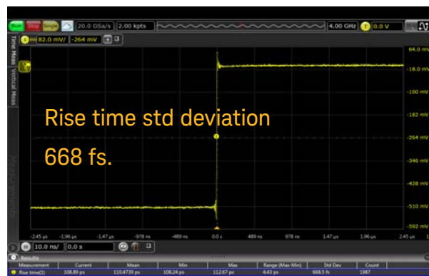
Figure 1(b). Note the difference in the standard deviation of rise time measurements. Both scopes are rated at 4 GHz bandwidth, are sampling at 20 GSa/s and set to the same settings. When measuring a fast rise time, the Infiniium S-Series reports a rise time value with standard deviation of 668 fs while the LeCroy scope reports a standard deviation of 4 ps, six times larger than the standard deviation measured by the Infiniium S-Series. Small standard deviations when measuring rise time on the same signal indicate superior signal integrity and a better horizontal system.
