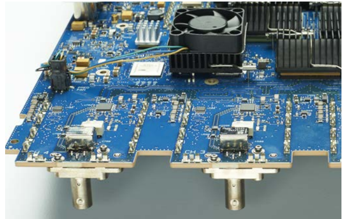
Figure 5. Infiniium S-Series oscilloscopes include a new low-noise front end designed as a companion to the 10-bit ADC, that reduces noise by 2x.
