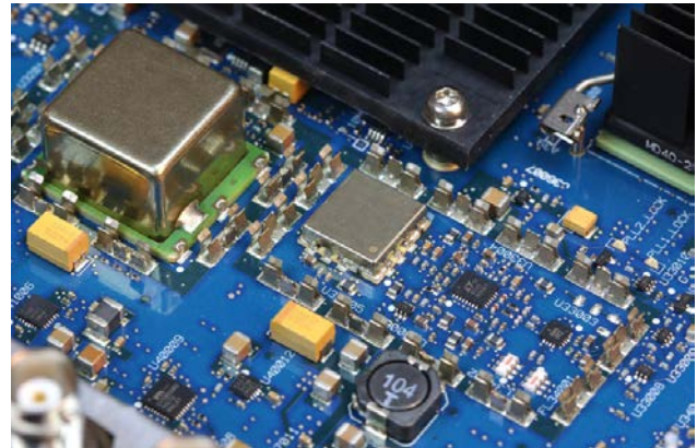
Figure 11. Infiniium S-Series oscilloscopes include a new time base technology block. It's clock accuracy is an impressive 75 parts per billion. Intrinsic jitter for short record lengths is less than 130 fs.
