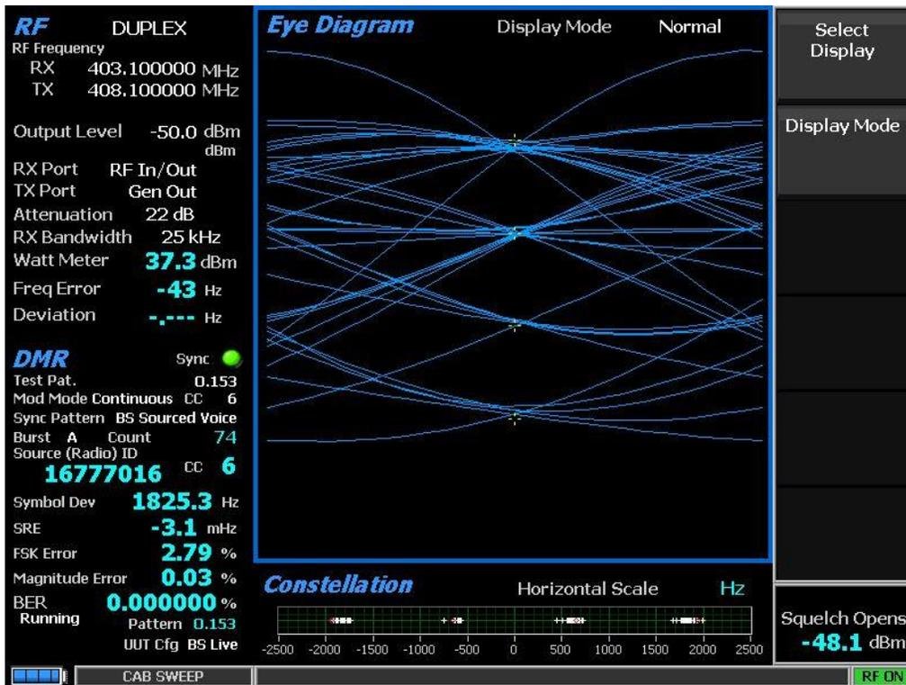
Figure 15 Live Repeater Mode with 0.153 BER
