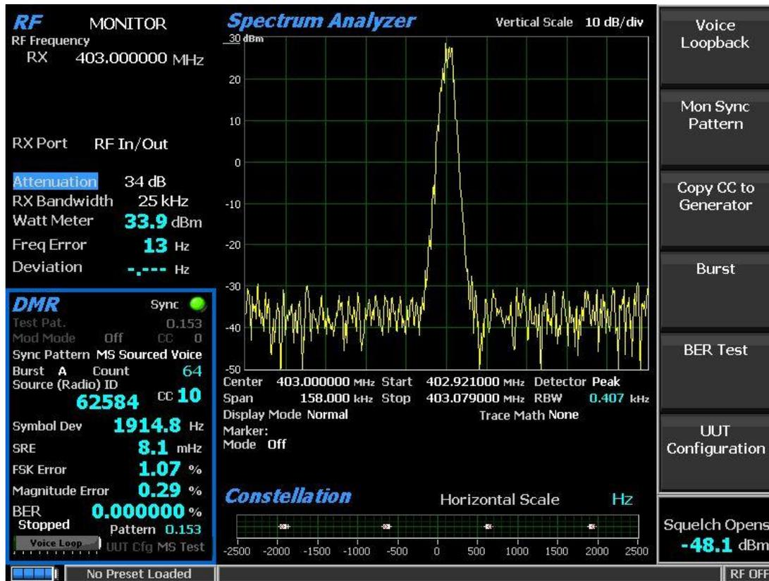
Figure 1 - DMR transmitter tests
