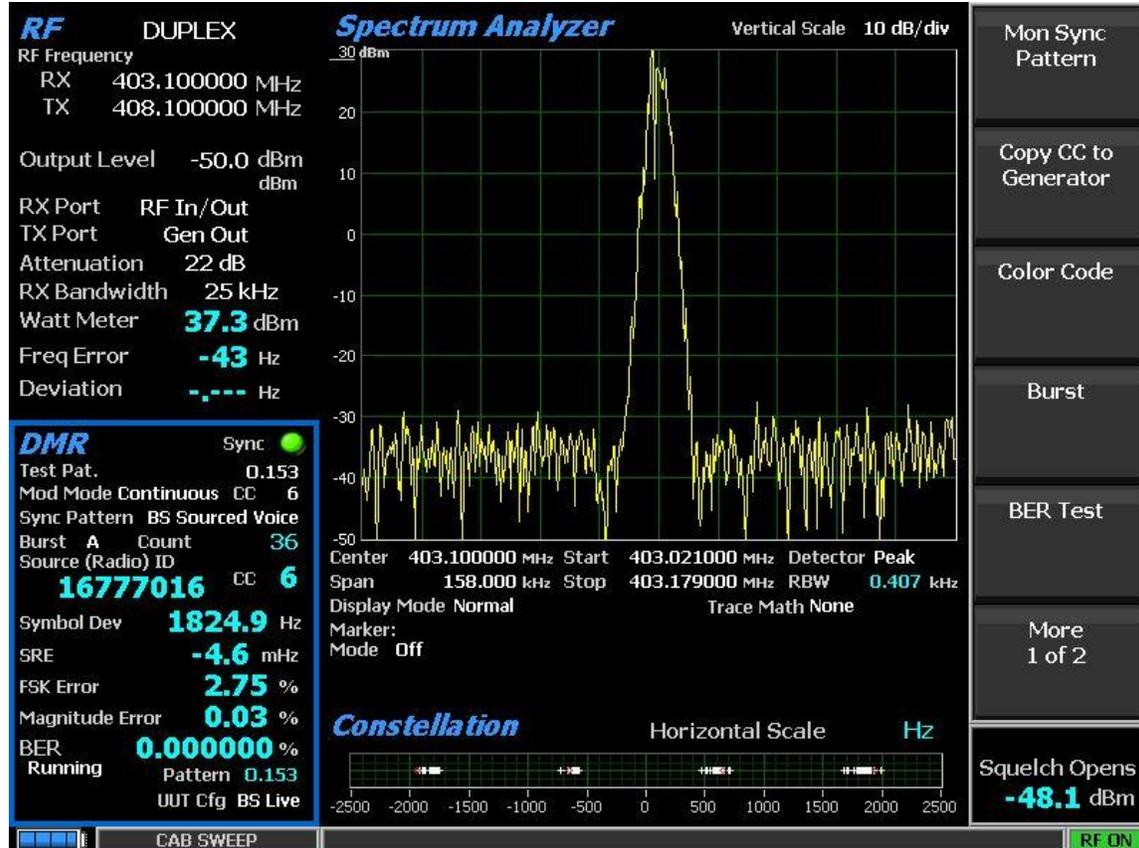
Figure 14 DMR Live mode in operation
