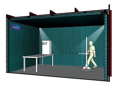
The Chronos 1F is designed to perform emission tests on automotive components. The design of the structure is optimised for maximum performances, in minimum space. The shielding and its pyramidal absorbers are manufactured by SIEPEL.
