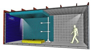
The Hera 3F is designed to perform pre-compliance emission and full compliance immunity tests at 3m distance on commercial equipment. The design of the structure is optimised for maximum performances, in minimum space. The shielding and its pyramidal absorbers are manufactured by SIEPEL.
