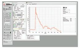
**PULSELab** software for pulsed waveforms acquisition, post-processing, display and report generation.
