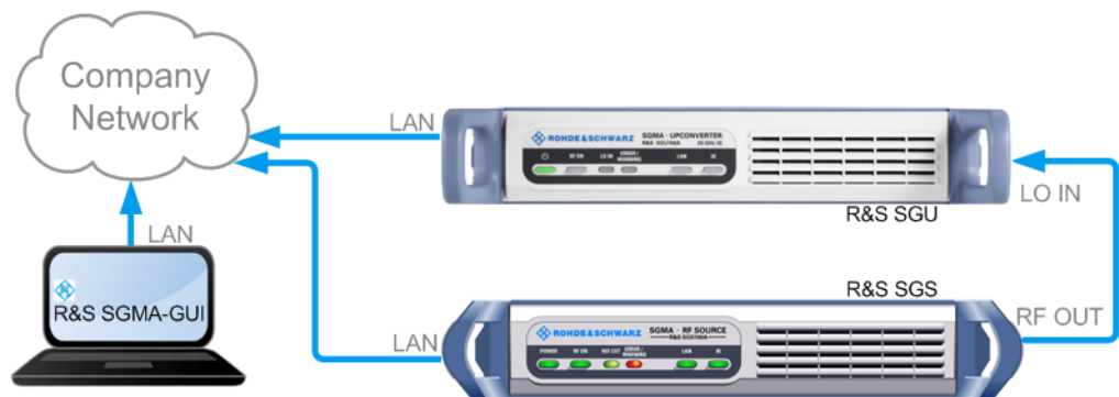
Figure 5-5: Connection of an R&S SGS and an R&S SGU in a company network
