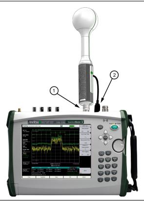
Figure 9-1. Connecting the Anritsu Isotropic Antenna
