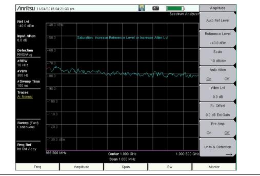
Figure 2-5. Saturation - Off Screen
