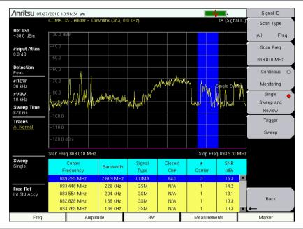
Figure 3-4. Interference Analyzer Signal ID, All Scan Type
