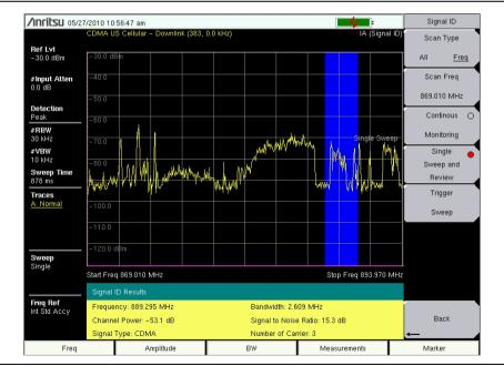
Figure 3-5. Interference Analyzer Signal ID, Freq Scan Type
