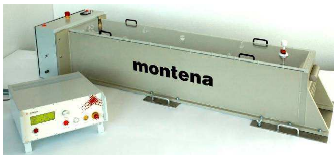
Fig. 3: Marx + peaking 360 kV pulse generator
