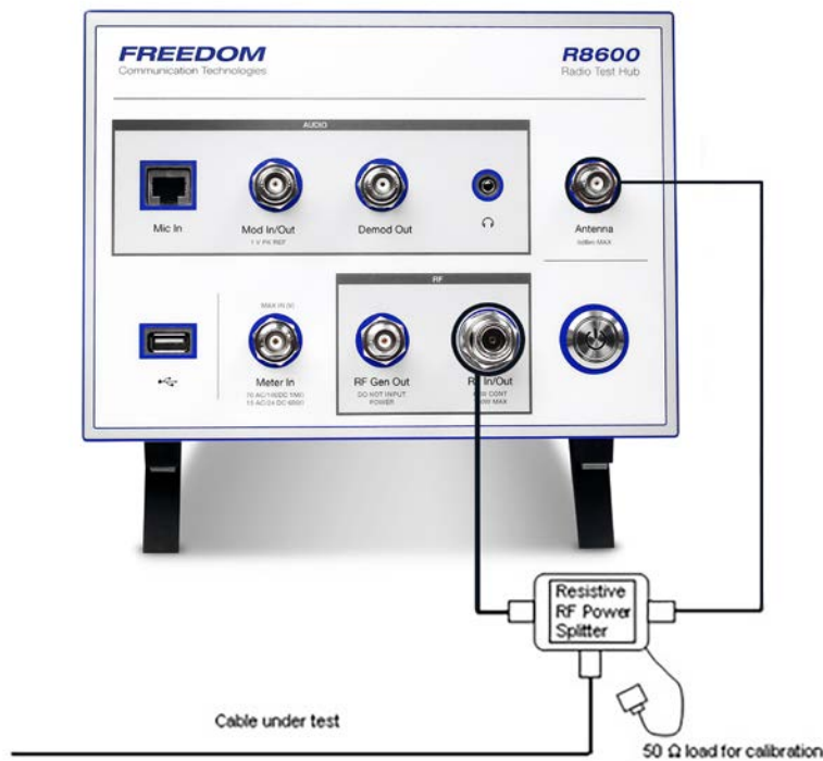
Figure 5.3-1 Connections for Cable Fault testing
