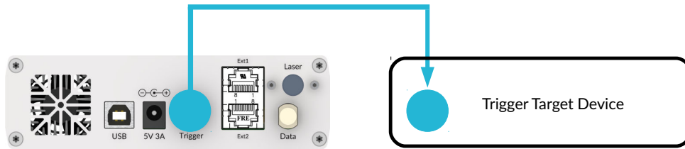
Figure 12: External trigger output using BNC connector
