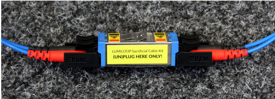
Figure 19: E2000 coupler of sacrificial optical cable assembly
