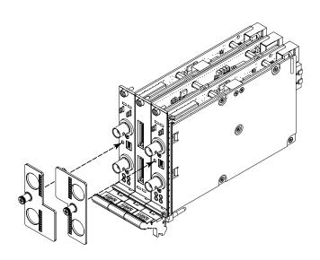
When the M9240A AutoProbe power module faceplates are connected, the oscilloscope input channels have AutoProbe interface connectors.
