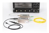
The two input electric signals are conditioned, digitalized and multiplexed into one optical signal in the transmitter module and sent to the receiver module through a single mode fibre. The receiver module converts back the optical signal in two electric signals.
