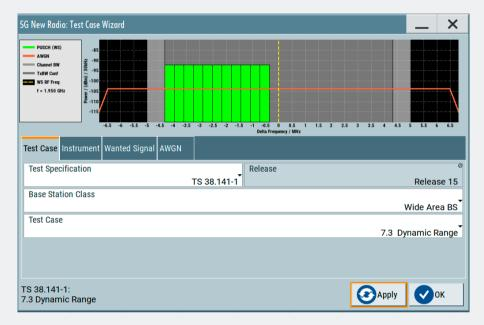
The 5G NR test case wizard allows the R&S<sup>®</sup>SMM100A to be conveniently and cleverly configured for BTS tests in line with 3GPP TS 38.141
