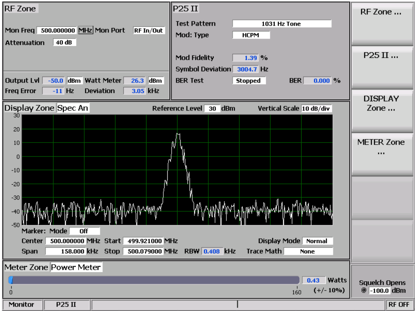
Figure 3.2.8.10.1-1 Main screen in Monitor Mode after selecting the P25 II Test Mode
