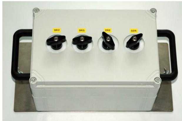
Figure 8 : Picture of termination resistor box TLB4
