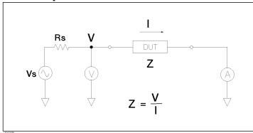
Figure E-1 illustrates the circuit model of impedance measurement using the E4981A. Vs is the measurement power supply voltage, and Rs is the output resistance of the E4981A. When voltage applied to a DUT is V and current flowing through the DUT is I, impedance Z is expressed by the equation Z = V/I.
