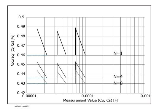
Figure 10-9Accuracy of Cp and Cs when measurement frequency is 1 MHz<br/>(measurement signal level: 1V)
