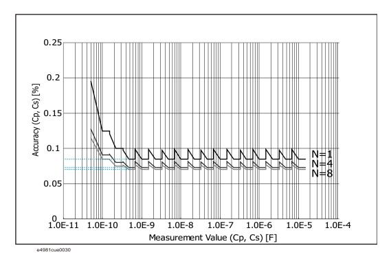
Figure 10-7Accuracy of D when measurement frequency is 1 kHz<br/>(measurement range: 22 µF to 100 µF / measurement signal level: 1V)
