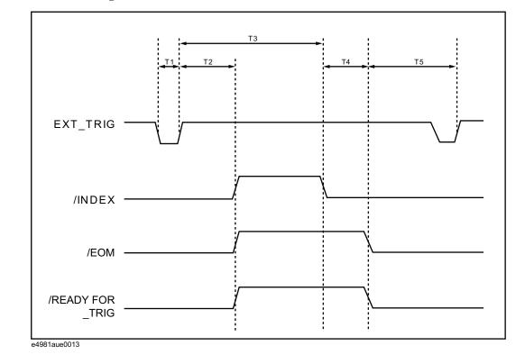
Figure 10-11 Timing chart and measurement time
