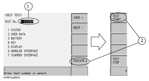
The following test items can be checked by using the self-test.
