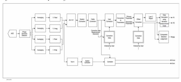
Figure 5-1 Data processing flow
