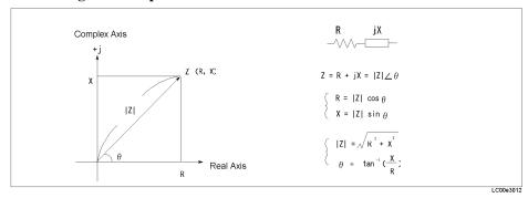
Figure E-2 Vector Diagram of Impedance
