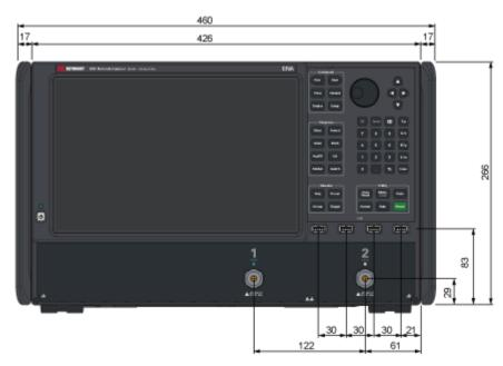
Dimensions (front view, E5080B with option 2P0 (1.85 mm), in millimeters)
