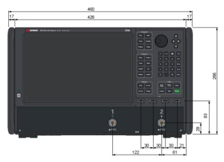
Dimensions (front view, E5080B with option 2M0/2N0 (2.4 mm), in millimeters)
