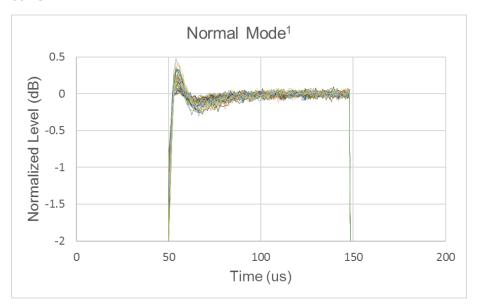
Measured with a 500 kHz IF bandwidth, averaging factor of 16 (Average Type = Point). With 100 us pulse width setting. 50 nsec/div.
