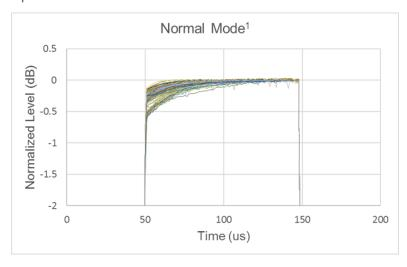
Measured with a 500 kHz IF bandwidth, no averaging (Average Type = Point). With 100 us pulse width setting. 50 usec/div.
