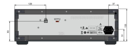
Dimensions (rear view, E5092A with option 020, in millimeters)
