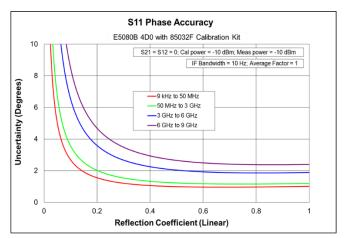
Table 3. Option 240/260/290/2D0/2K0/440/460/490/4D0/4K0/442/462/492/4D2/4K2 with bias tee options (Option 120 or 140) with 85032F Standard Mechanical Calibration Kit
