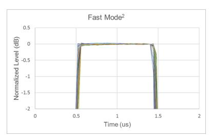
Measured with a 15 MHz IF bandwidth, averaging factor of 16 (Average Type = Point). With 1 us pulse width setting. 500 nsec/div
