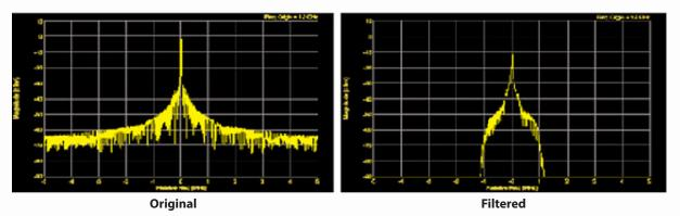
Apply bandpass filters to waveform segments with a 3-dB passband that is a selected percentage of the file's capture bandwidth.
