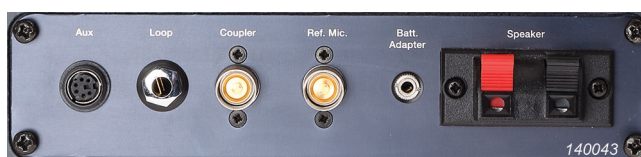
Fig. 2 All connections to the inside of the test box are made via the connectors on the back panel of Type 4232
