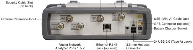
ALL CONNECTORS ARE CONVENIENTLY LOCATED ON THE TOP PANEL, LEAVING THE SIDES CLEAR FOR HANDHELD USE
