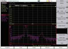
The VNA Mode in the VNA Master with standard Distance Domain allows simultaneous viewing of cable return loss and distance to fault.
