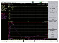
The VNA Master's 2-port analyzer provides simultaneous measurement of  $\rm S_{21}$  insertion loss and  $\rm S_{11}$  return loss.
