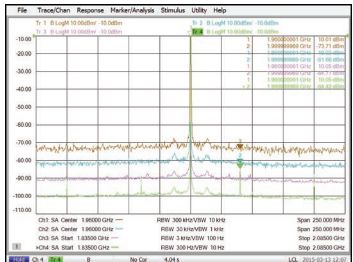
Above plot shows -84 dBm spurious measurements in the presence of a +10 dBm signal, with (from top to bottom) approximate S/N (at RBW) of 80 dB (300 kHz), 90 dB (30 kHz), 100 dB (3 kHz), and 110 dB (300 Hz)
